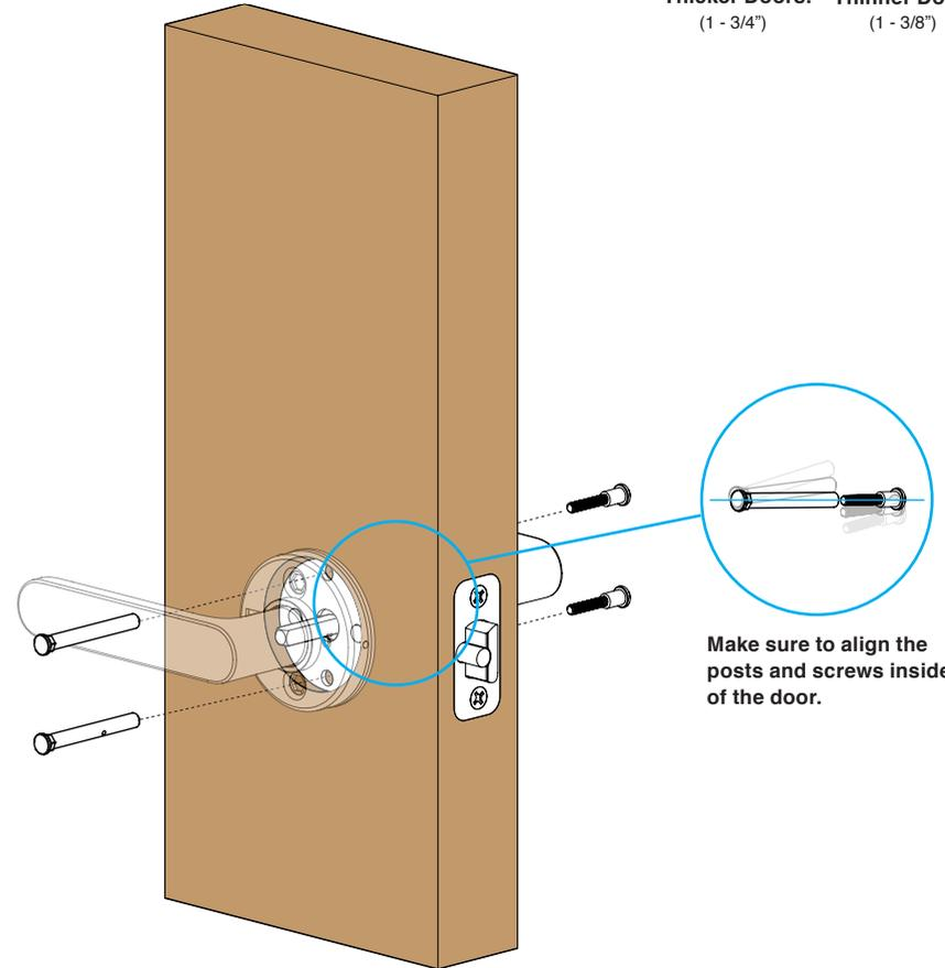
Make sure to align the posts and screws inside of the door.
