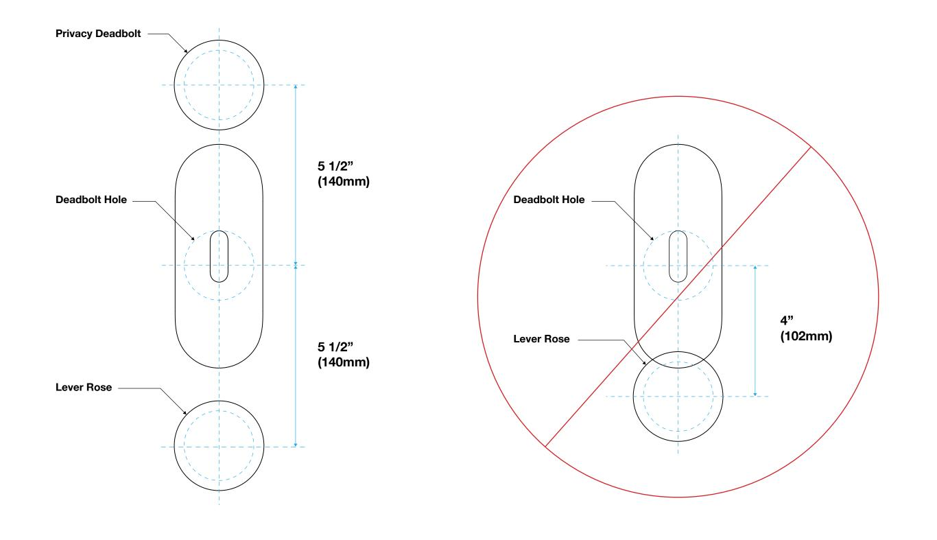
C2 must be at a 5.5" center-to-center spacing from the lever set bore hole. A privacy deadbolt can be installed above C2 at a 5.5" center-to-center bore hole spacing.
